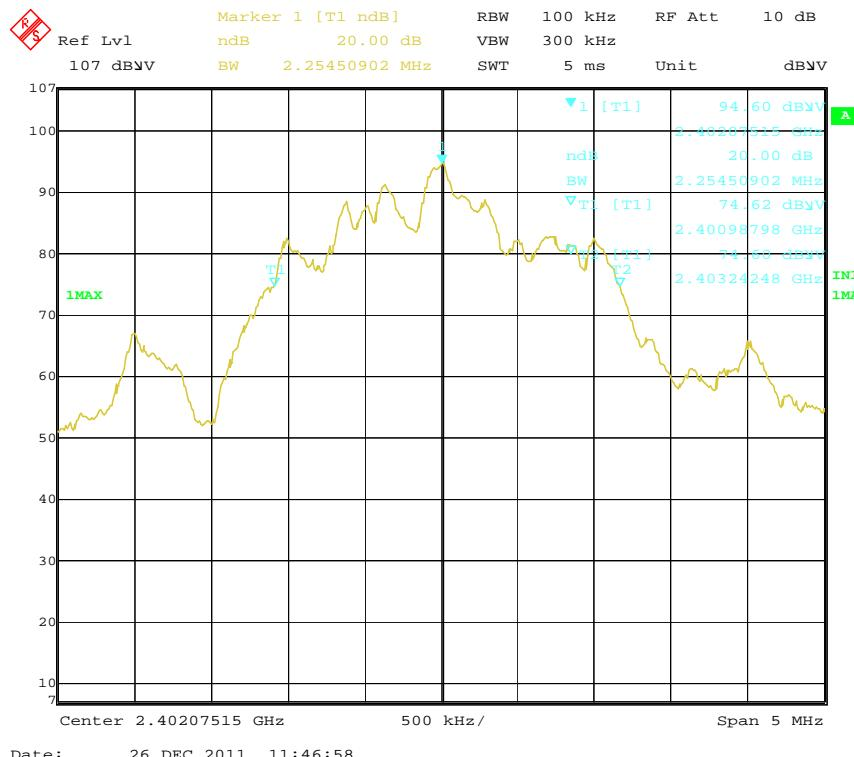
Measurement Result @The Channel 2440MHz
