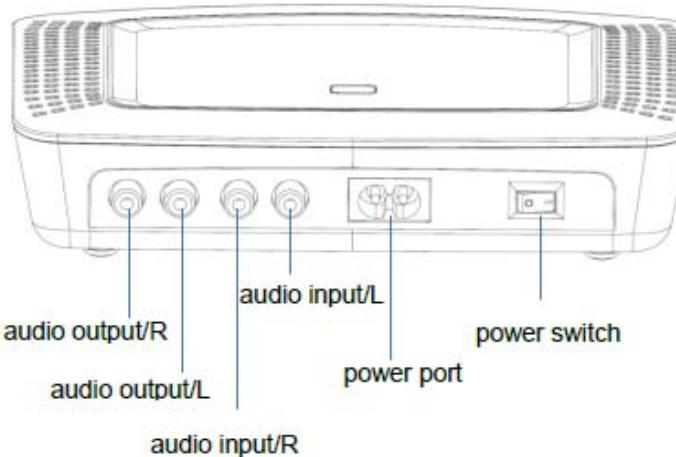
During using, the audio-input port can be connected with the PC, DVD and some other media player devices. All these audio signals will be output together with the voice from the microphone.
