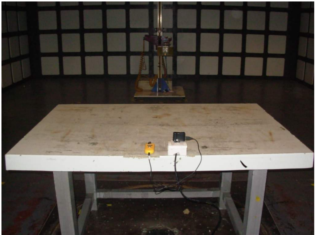
BACK VIEW OF RADIATED EMISSION TEST (ABOVE 1GHz, LYING DIRECTION)
