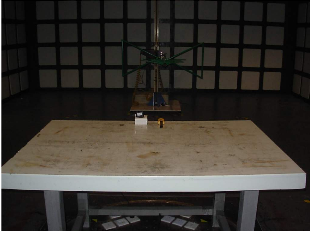
FRONT VIEW OF RADIATED EMISSION TEST (BELOW 1GHz, LYING DIRECTION)
