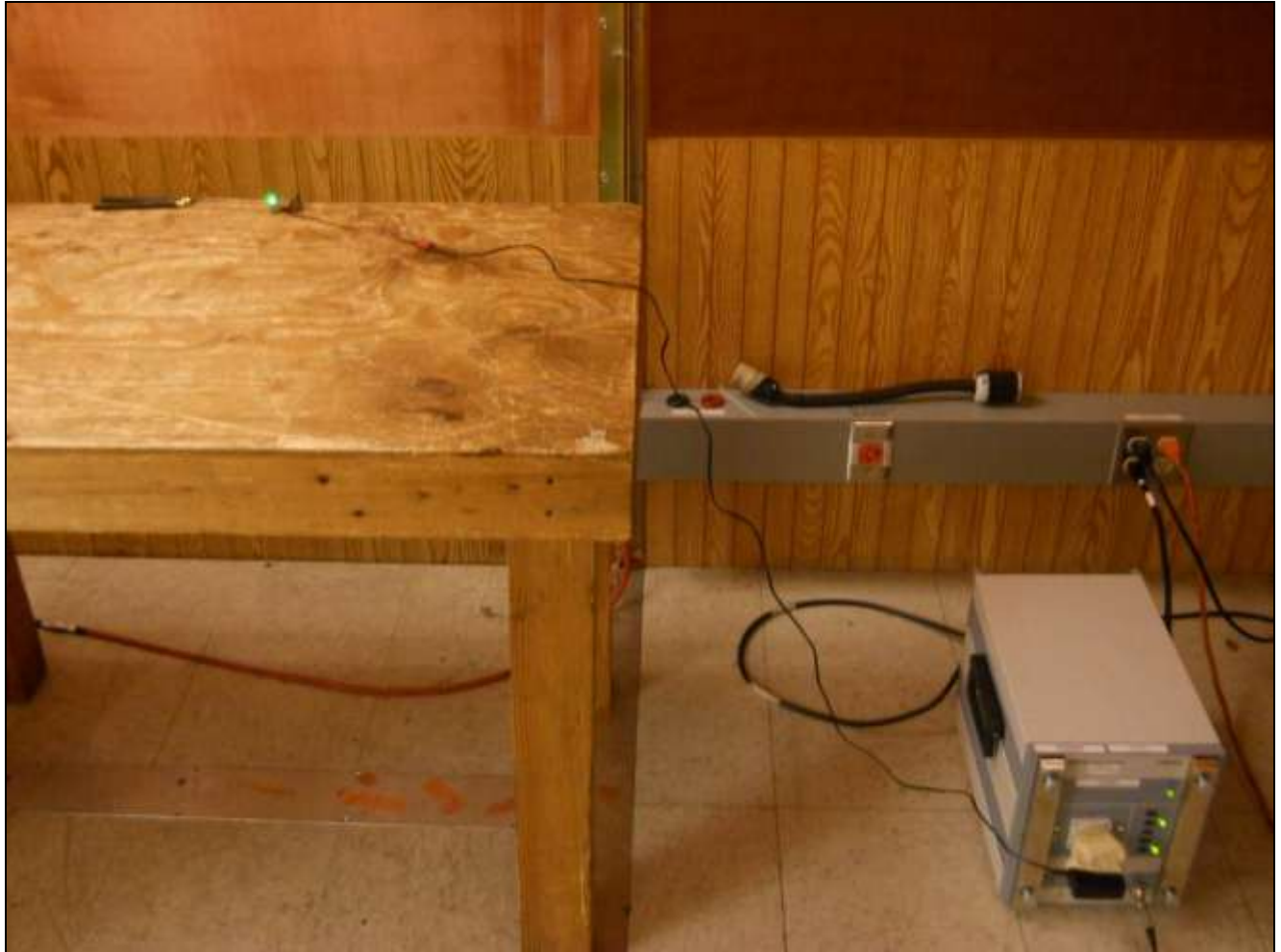
Photograph 1. Conducted Emissions, Test Setup
