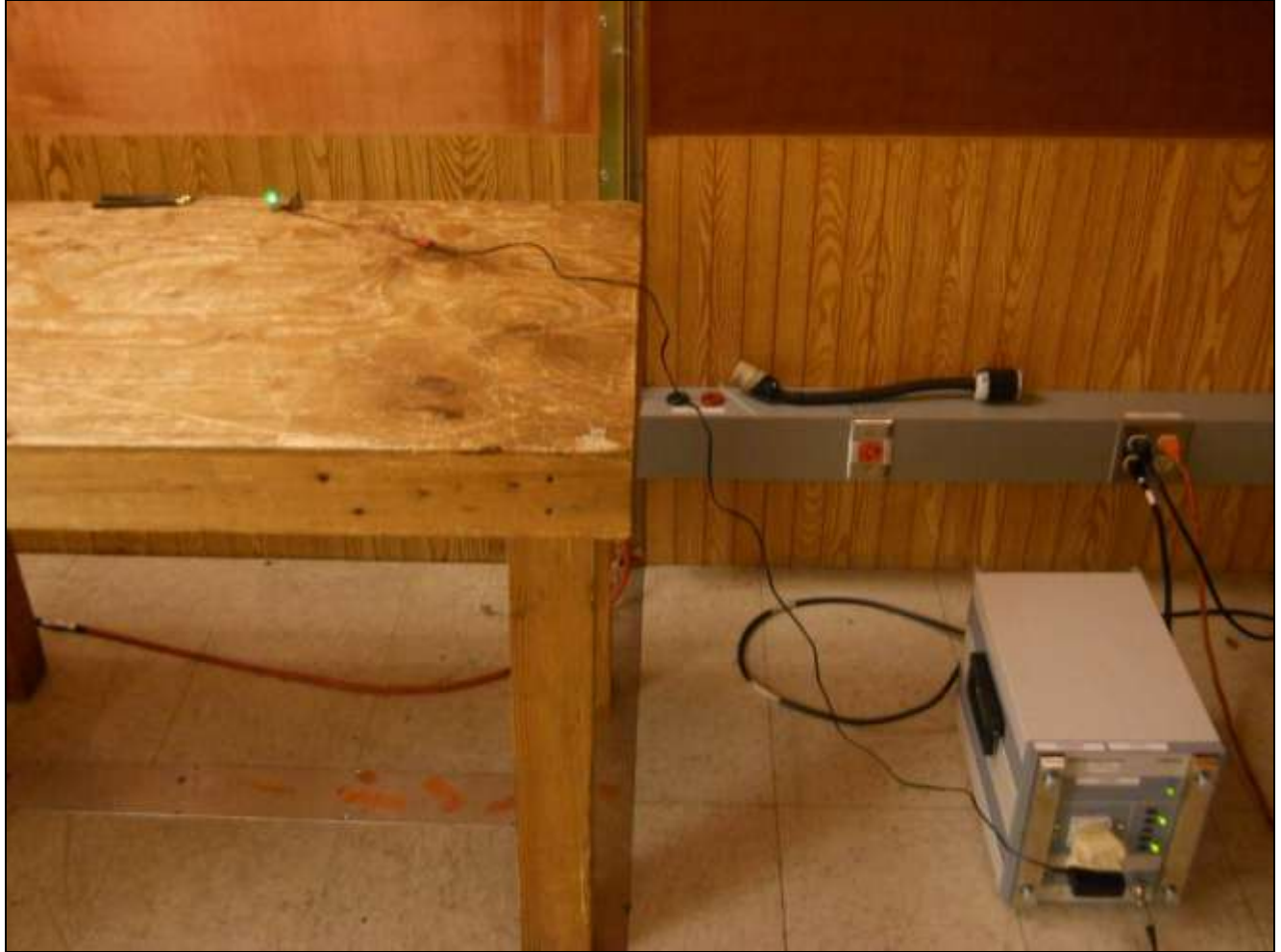
Photograph 2. Conducted Emissions, 15.207(a), Test Setup
