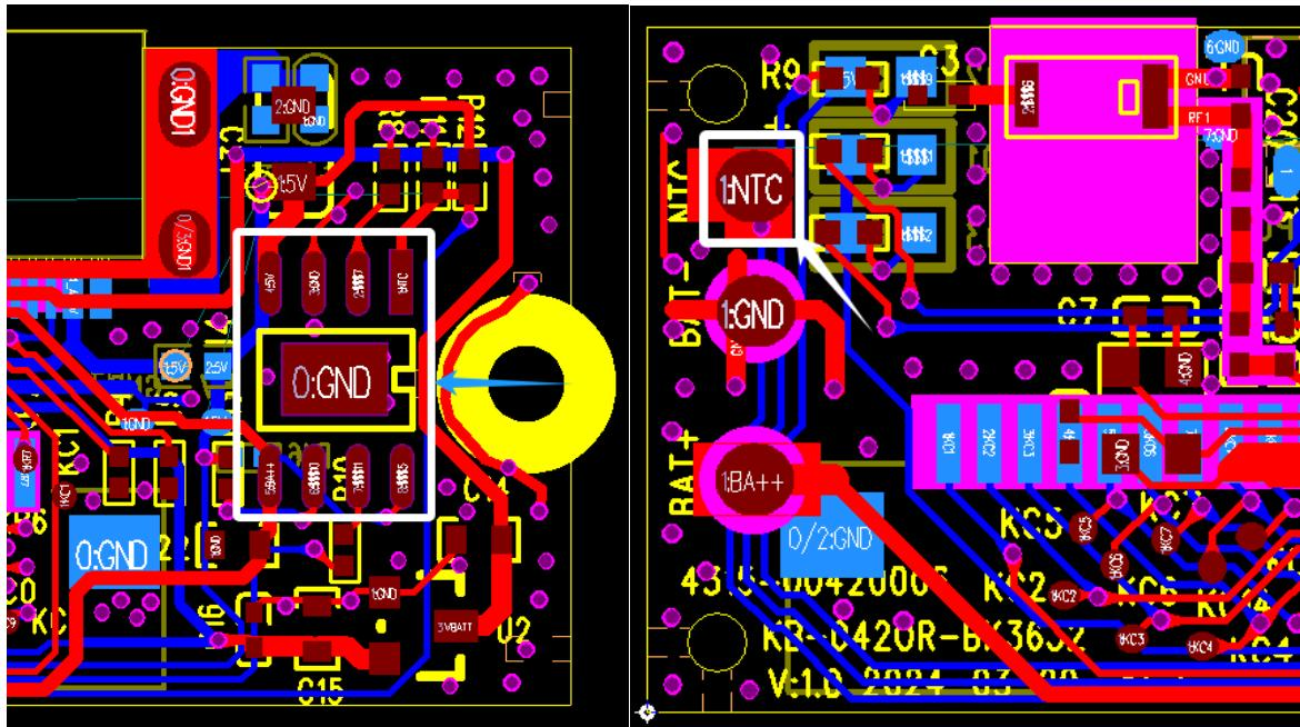
3. R8 from 4.7K to 5.1K; R10 from 0Ω to 10KΩ; add R16 (1KΩ); add R11 (130KΩ); add R12(5.6KΩ); add R13 (10KΩ); add R14 (0Ω) , necessary peripheral circuits for matching the new charging management IC;
