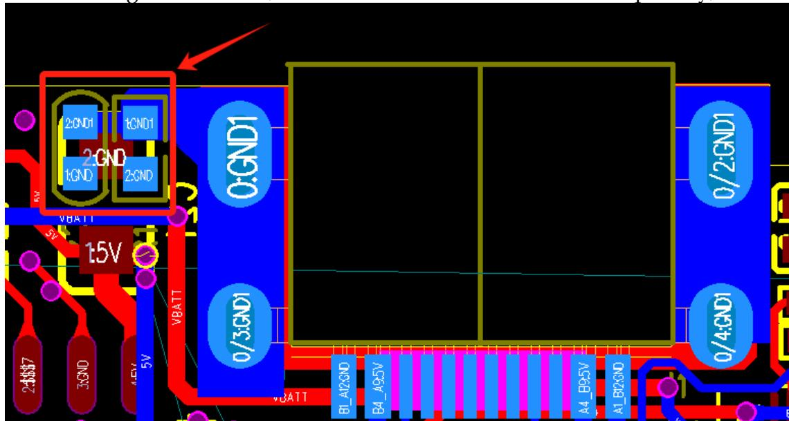
2. The charging management IC\_U4 changed from SS4054 to CE3221; an NTC thermistor (10K $\Omega$  B=3435) was added to the protection board of the lithium battery, and a wire was led out to connect to the PCB, so that the keyboard had high and low temperature charging protection function;
