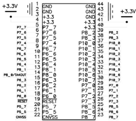
All the GPIO from the Renesas M16C/6B3 are available on the module pinout.
