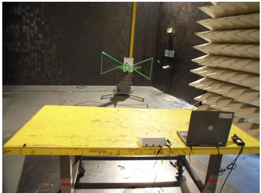
**For radiated emissions above 1GHz****FRONT VIEW**
