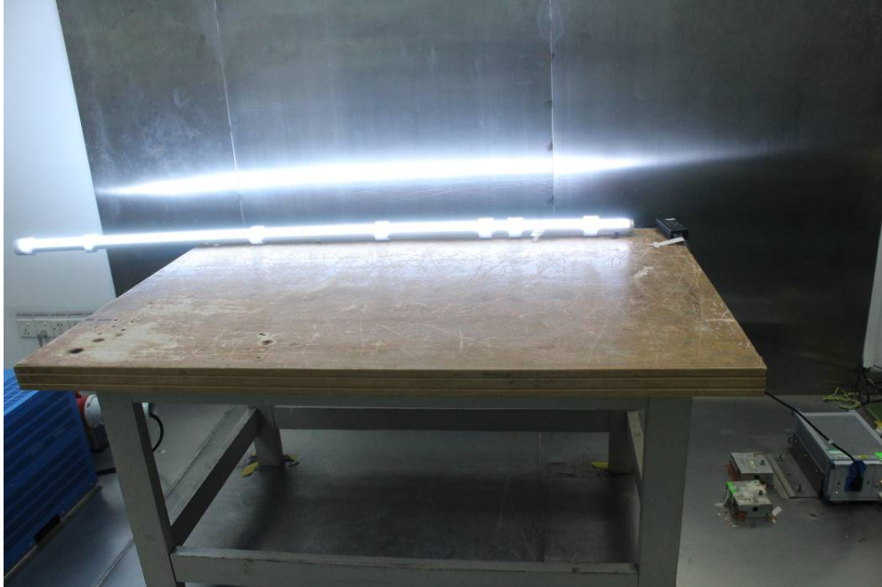
Conducted Emissions - Front View
