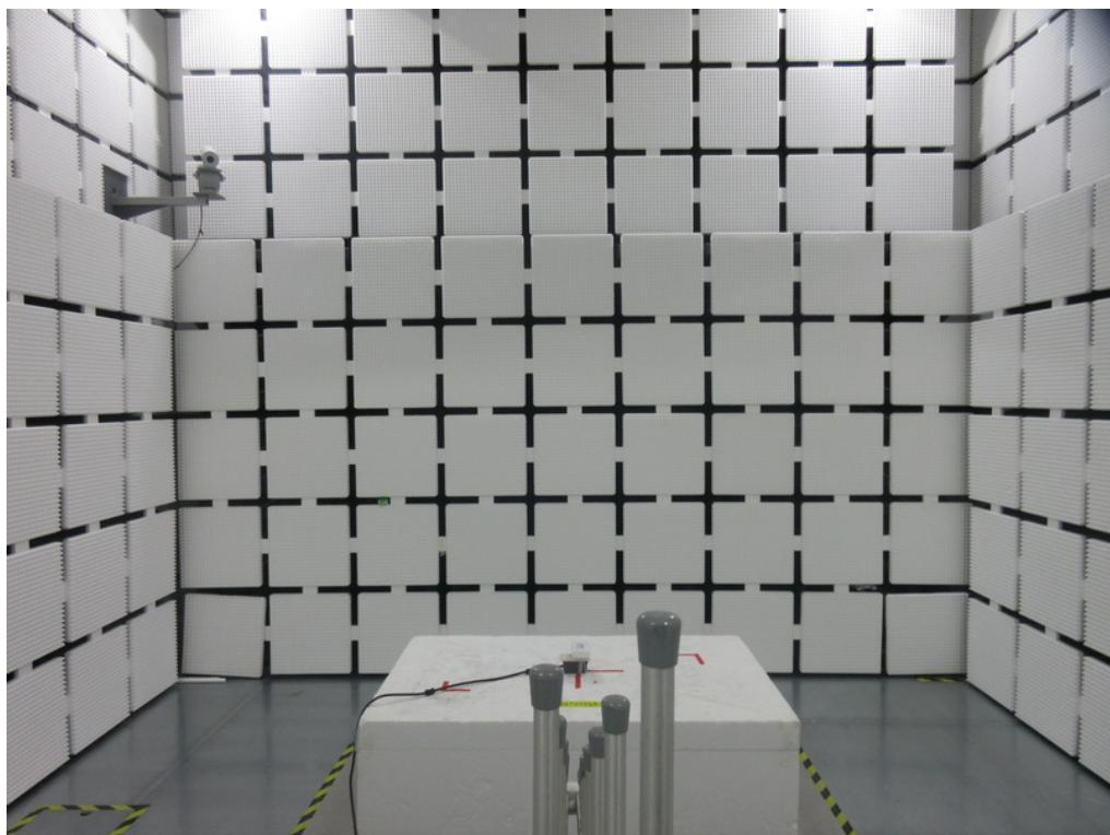
**Radiated Emissions Test Photos****Above 1 GHz**
