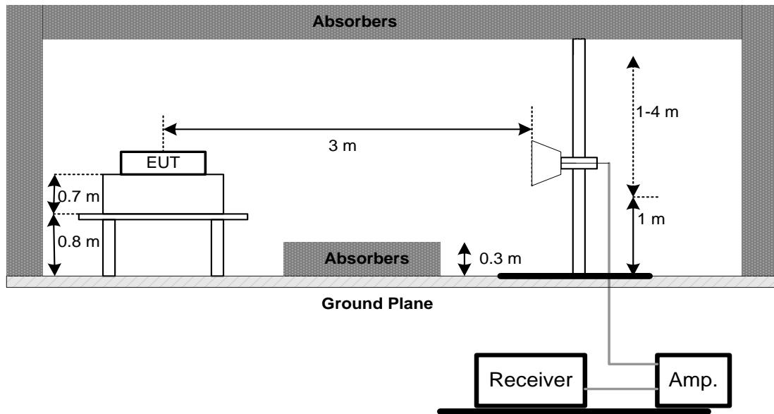
(C) For Radiated Emissions Below 30MHz
