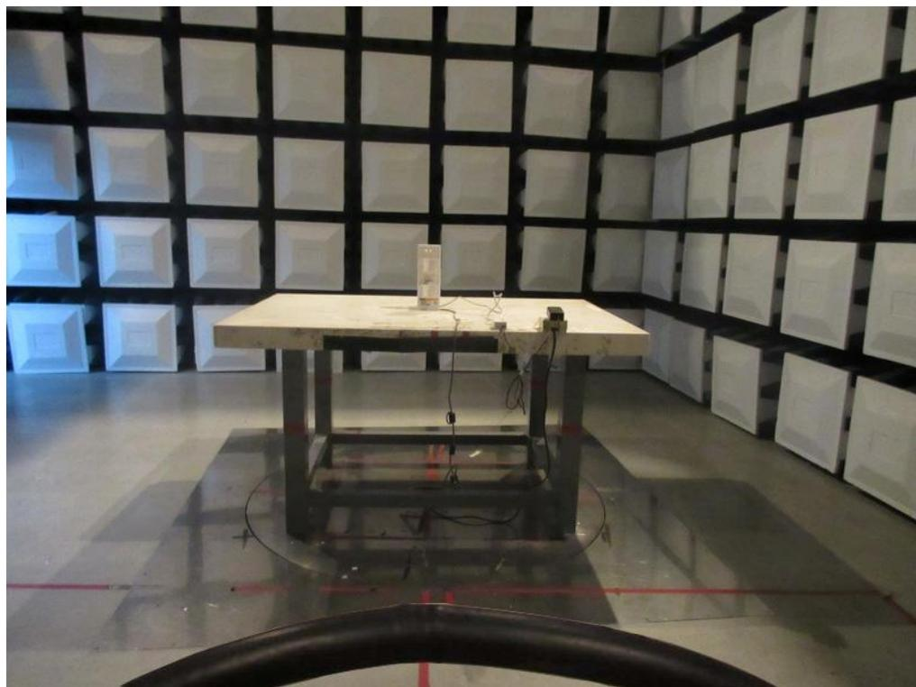
**Radiated Measurement Photos-Internal Antenna****30MHz to 1000MHz**
