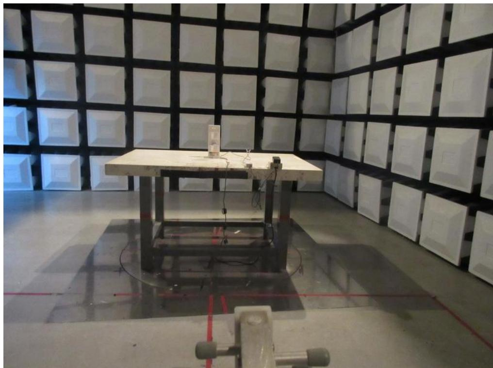
**Radiated Measurement Photos-Internal Antenna****Above 1000MHz**
