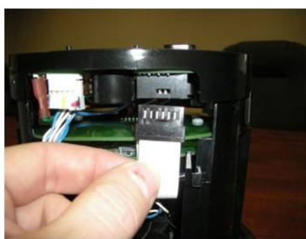
Figure 16 Attach White Ribbon
