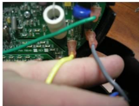
Figure 12 Locate Power Leads Yellow/Gray
