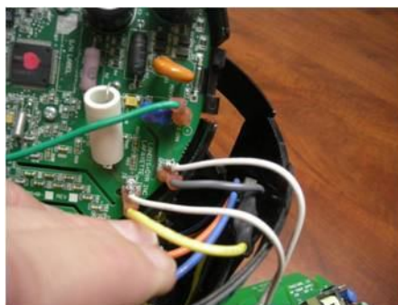
Figure 14 Re-Connect Yellow/Gray Leads
