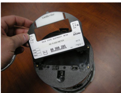
Figure 2 Lift Label Cover
