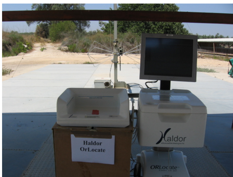
Figure 3. Radiated Emission Test 30 MHz- 1000 MHz
