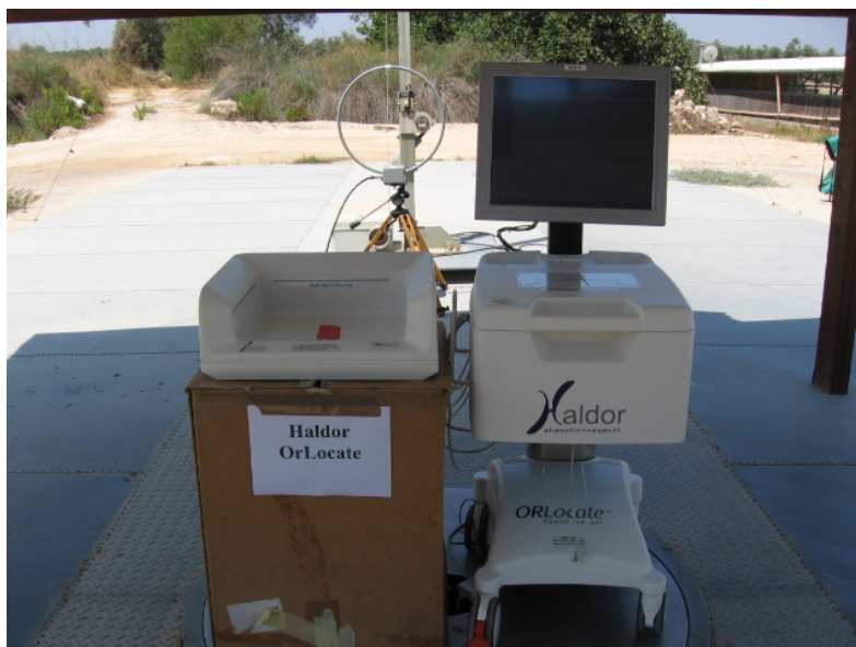
Figure 2. Radiated Emission Test 9 kHz- 30 MHz
