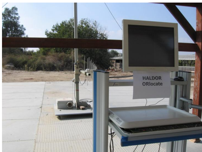
Figure 10. Radiated Emission Test 300MHz-1000MHz Flat Antenna
