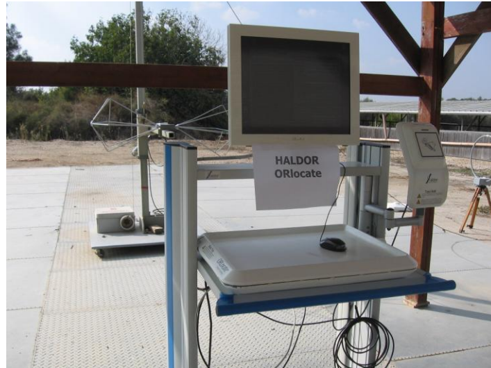
Figure 7. Radiated Emission Test 30MHz-300MHz Tool Add
