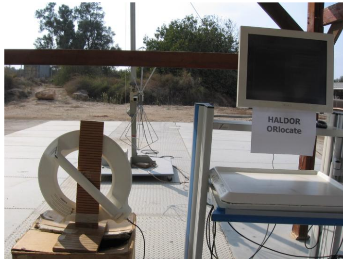
Figure 8. Radiated Emission Test 30MHz-300MHz Locator
