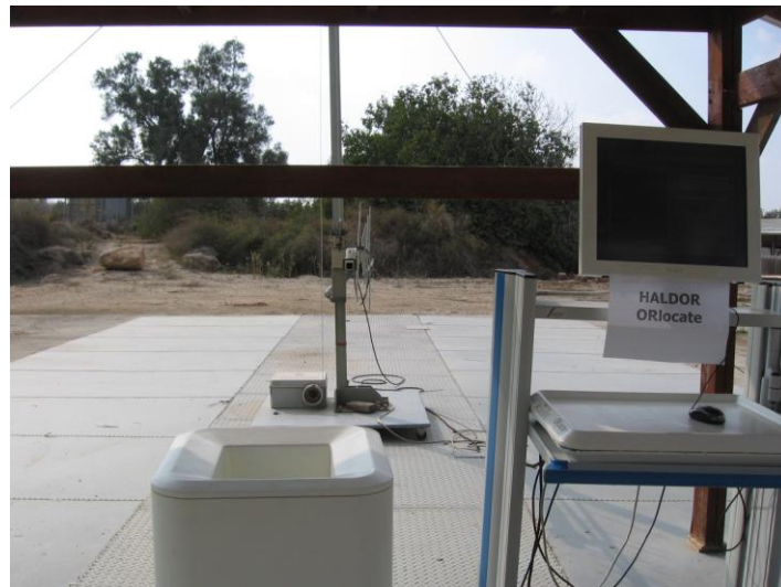
Figure 5. Radiated Emission Test 9kHz-30MHz Sponge Bucket
