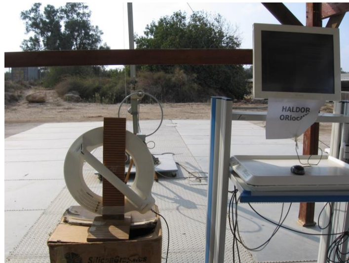
Figure 4. Radiated Emission Test 9kHz-30MHz Locator
