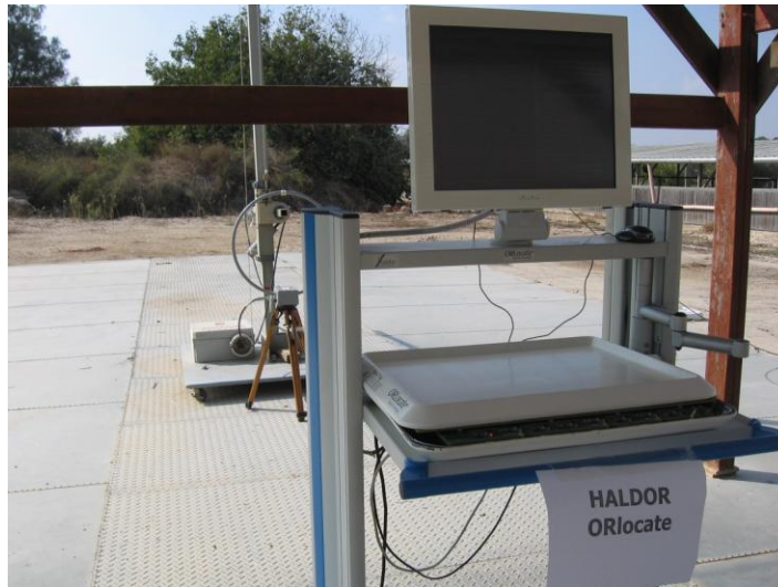
Figure 2. Radiated Emission Test 9kHz-30MHz Flat Antenna
