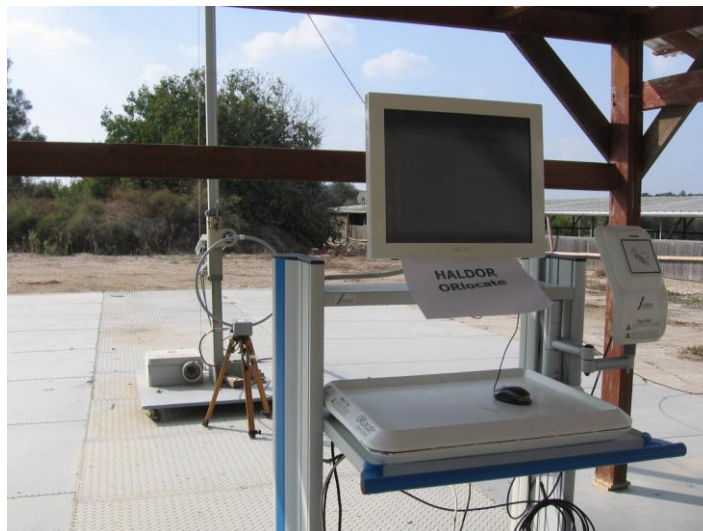
Figure 3. Radiated Emission Test 9kHz-30MHz Tool Add
