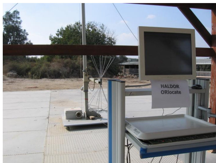
Figure 6. Radiated Emission Test 30MHz-300MHz Flat Antenna
