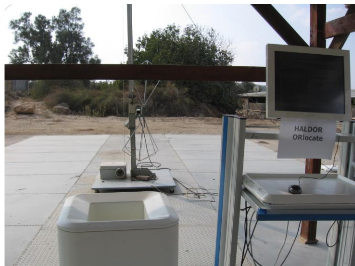
Figure 9. Radiated Emission Test 30MHz-300MHz Sponge Bucket
