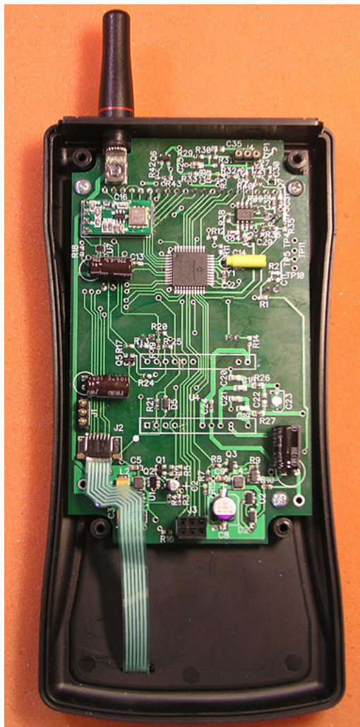
P.C Board mounted in front cover (scale: 1:1.5)
