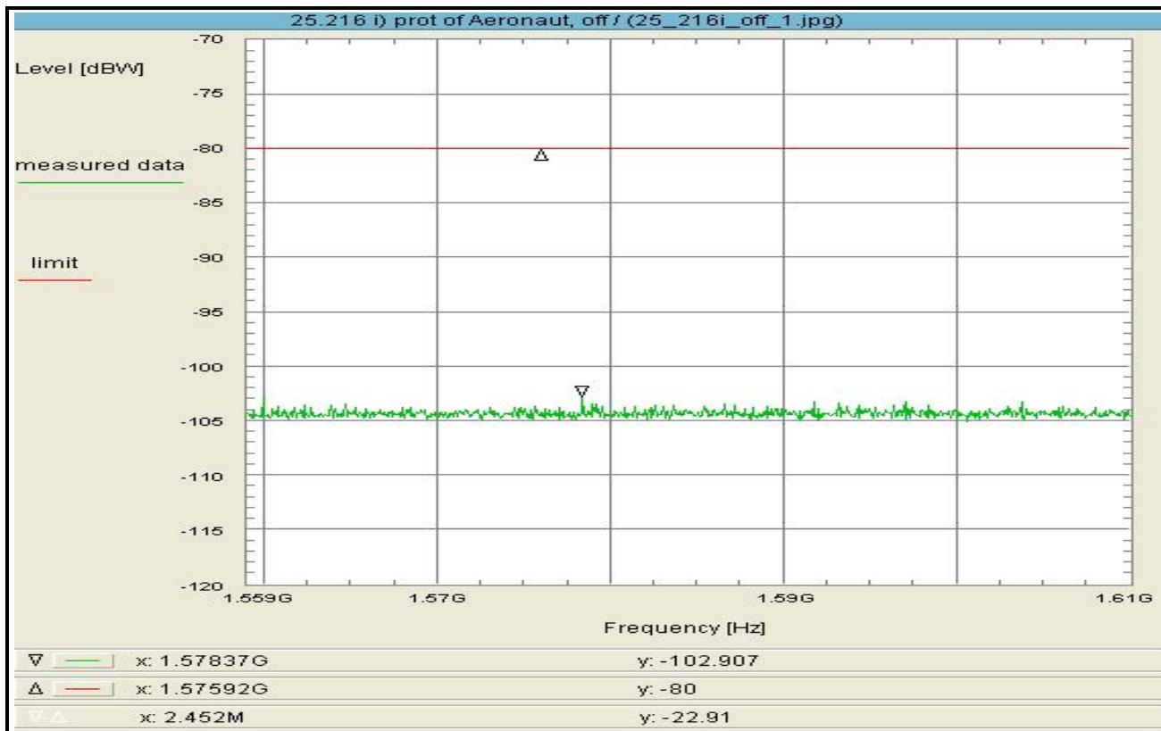
Subclause: 25.216 i) Limits on emissions from mobile earth stations for protection of aeronautical radionavigation-satellite service
