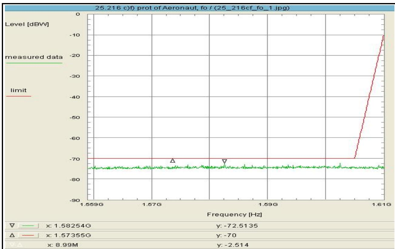
Subclause: 25.216 c)f) Limits on emissions from mobile earth stations for protection of aeronautical radionavigation-satellite service
