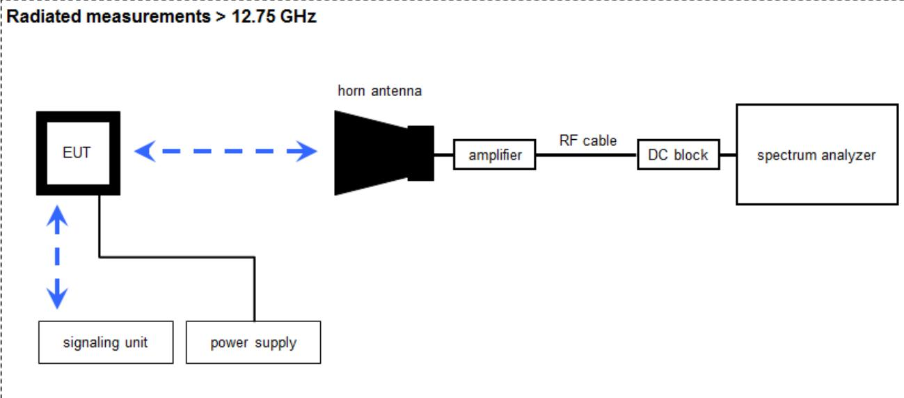
Measurement distance: horn antenna 25 cm
