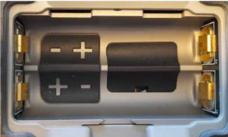
Photo: Battery compartment contacts identification
