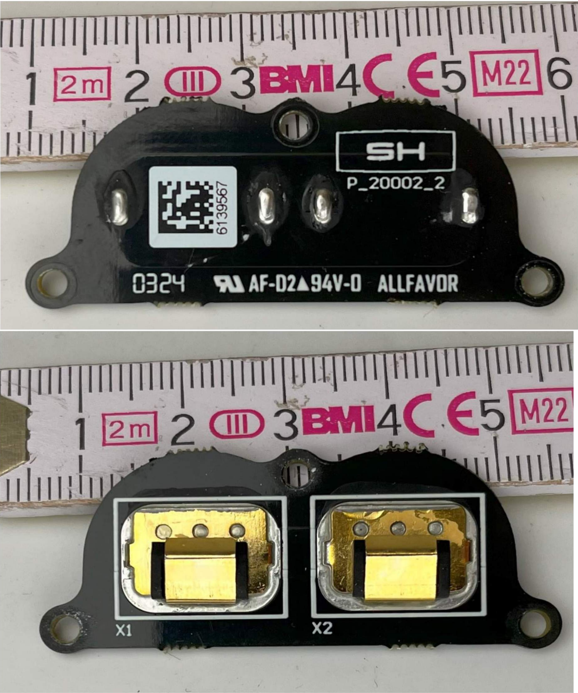
Battery contact board:
