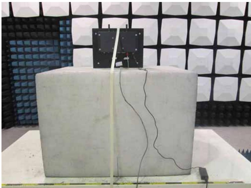
**ANTENNA PORT CONDUCTED RF MEASUREMENT SETUP**
