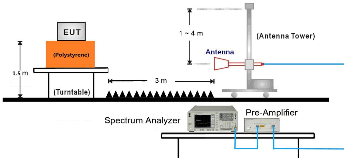
18GHz ~40GHz Test Setup:
