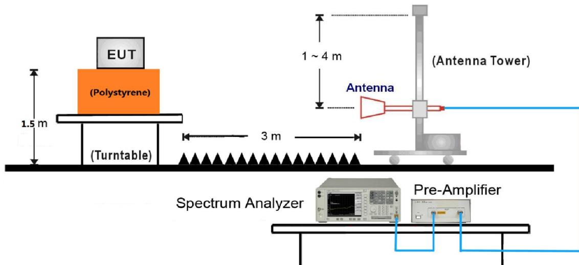
18GHz ~40GHz Test Setup:
