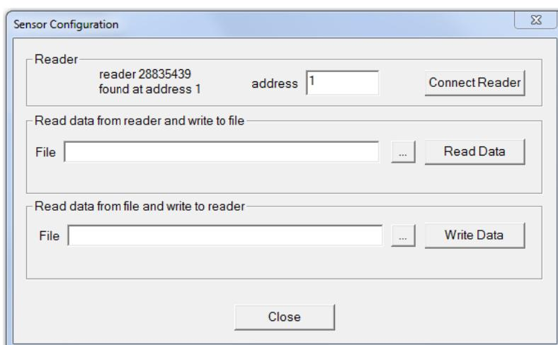
For the 12 sensor system the sensor configuration is provided in the file “12sensors\_3.spf” using Sensor ID [11] – [22] at Antenna 1.
