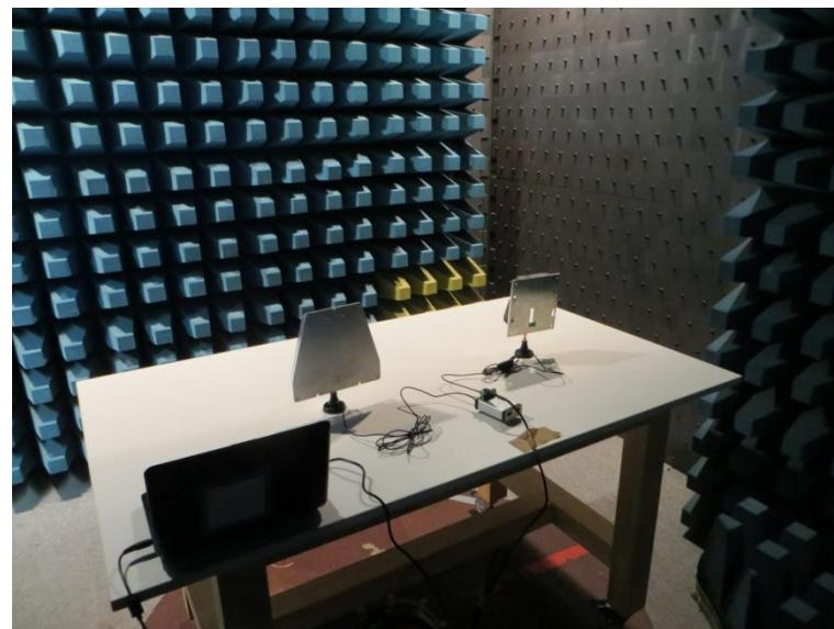
**Test setup for radiated emission measurement
