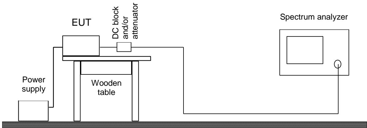
Test instruments used for conducted measurements:
