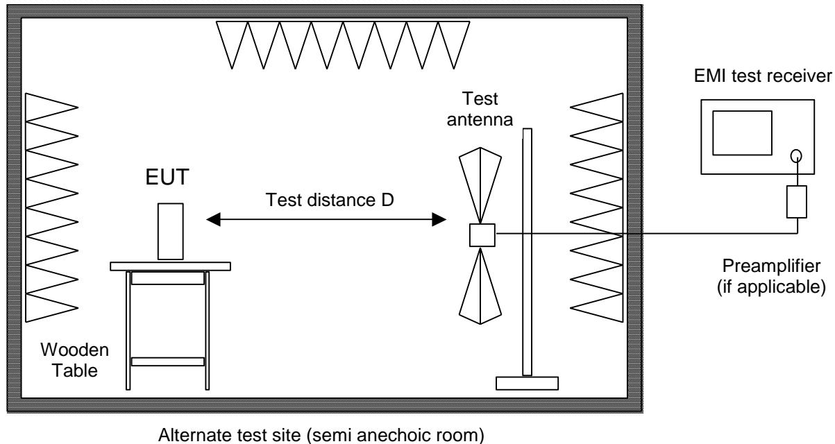
Alternate test site (semi anechoic room)
