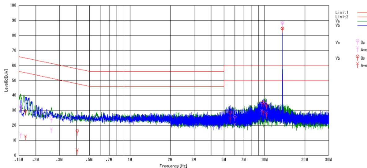
**AC Power line conducted emission. (Antenna was terminated)****Regulated DC power supply AC port**
