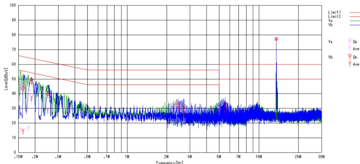
**AC Power line conducted emission. (Antenna was terminated)
