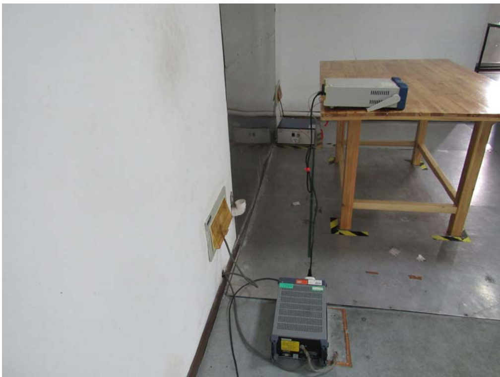
Conducted Emissions Setup Side View
