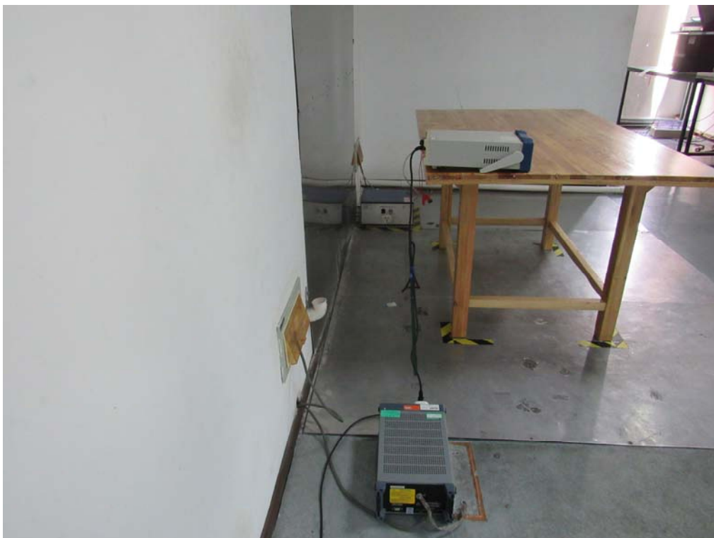
Conducted Emissions Setup Side View
