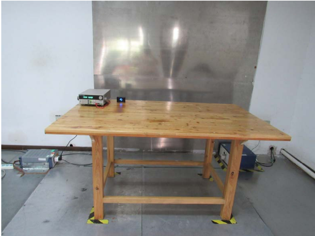
Conducted Emissions Setup Front View
