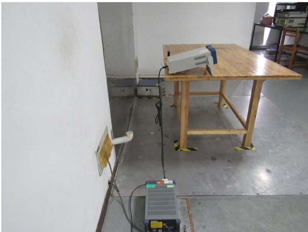
Conducted Emissions Setup Side View
