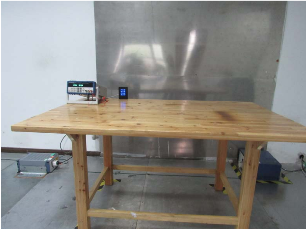
Conducted Emissions Setup Front View
