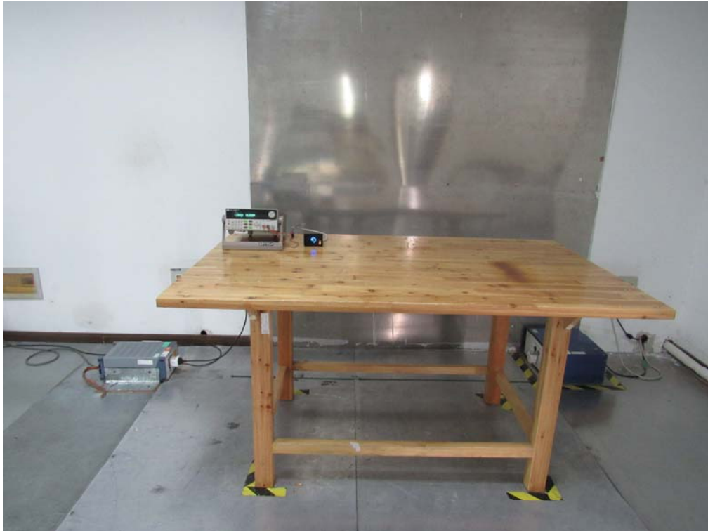
Conducted Emissions Setup Front View
