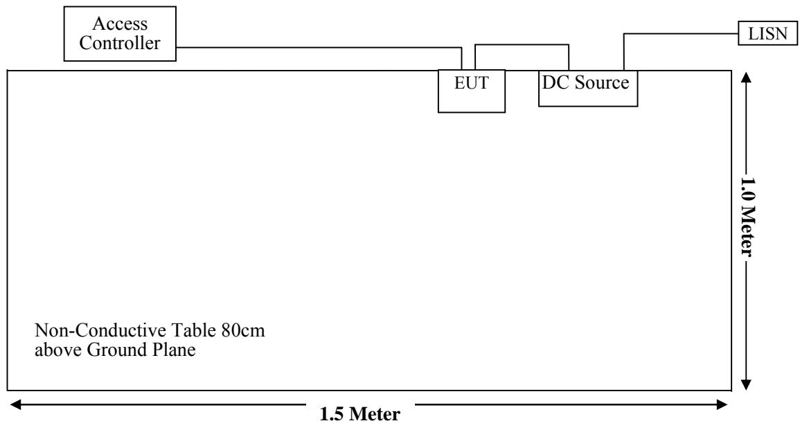
For Radiated Emissions (Below 30 MHz):
