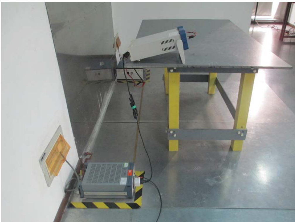
Conducted Emissions Test Setup Side View
