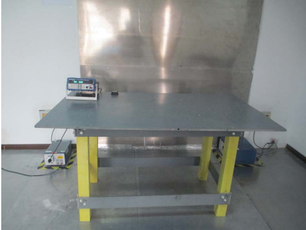
Conducted Emissions Test Setup Front View
