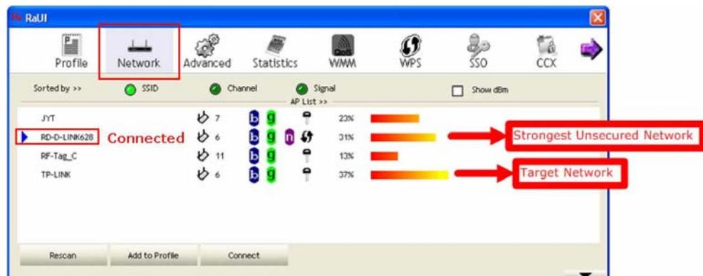
To join your target network, in Network tab, click on target network then **Connect**. Choose the security type of your network and type your security key, click on **OK** to complete a basic network connection.
