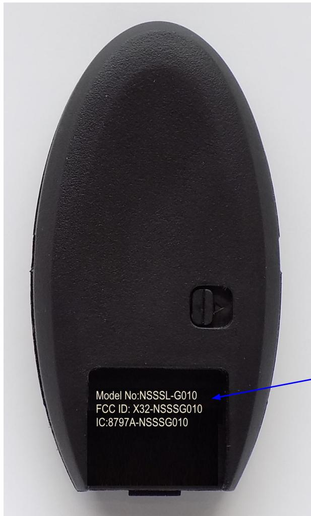
The FCC/IC label is located on the back of the remote shell beneath the emergency key.
