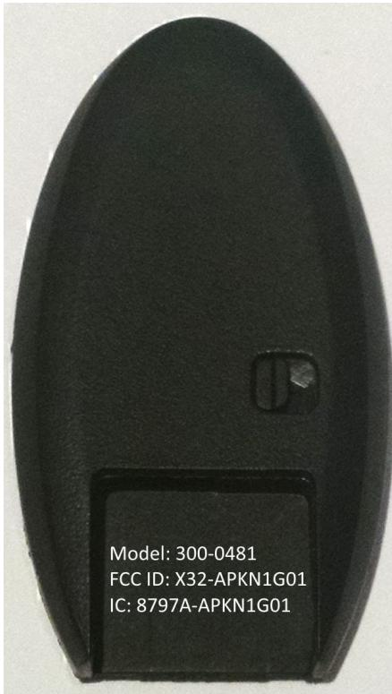
The FCC/IC label is located on the back of the remote shell beneath the emergency key.
