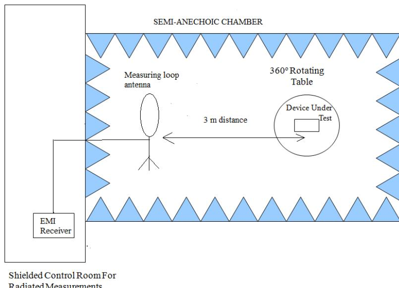
Radiated measurements setup  $f > 30$  MHz:
