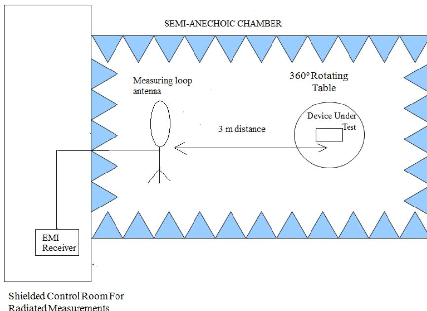
Radiated measurements setup from 30 MHz to 1 GHz:
