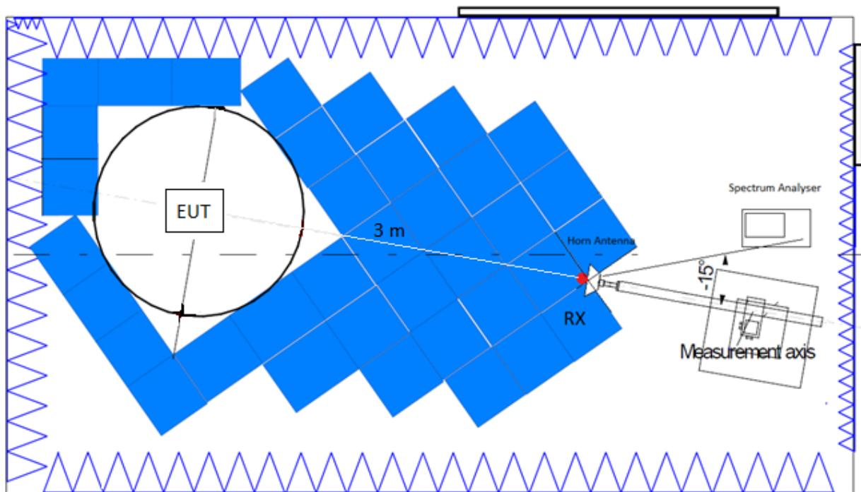
Radiated measurements setup  $f > 17$  GHz:
