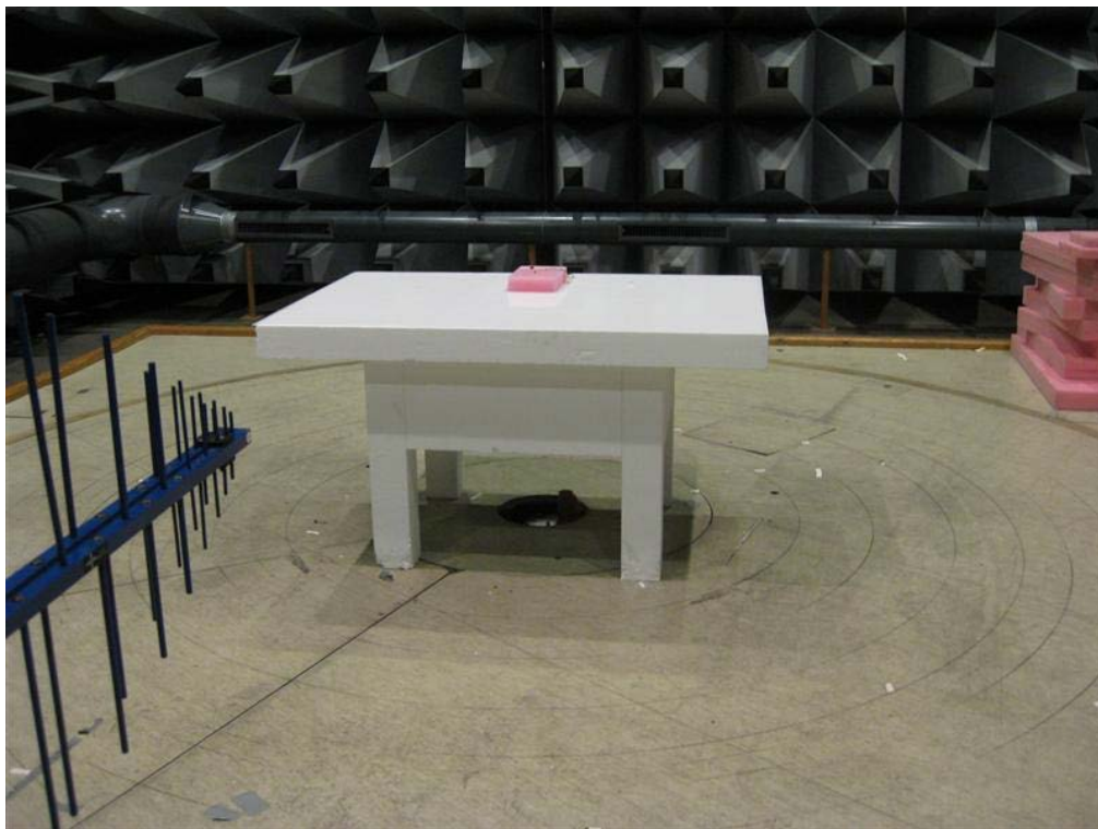
Photo 4.4.1 Test setup regarding measurement of radiated emission below 1 GHz.
