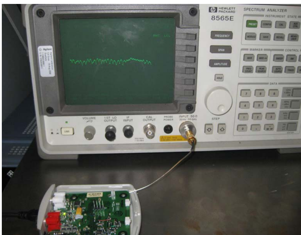
Photo 4.9.2 Test setup regarding measurement of power spectral density.
