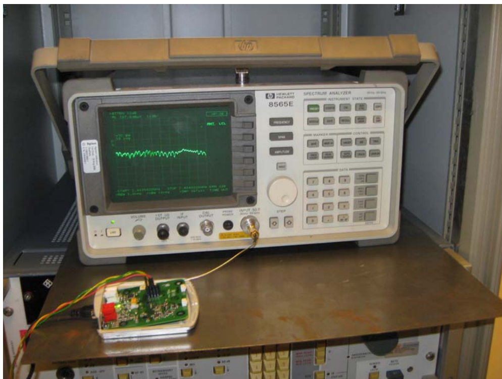
Photo 4.9.1 Test setup regarding measurement of power spectral density.
