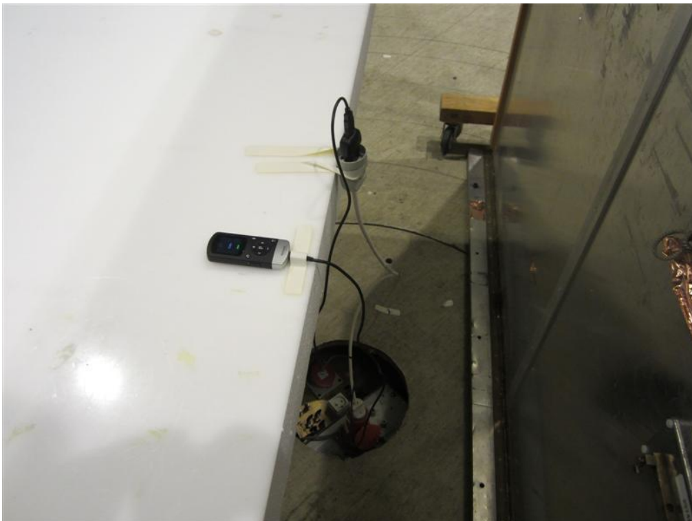
Photo 4.2.2 Test setup regarding measurement of radio frequency voltage on mains.
