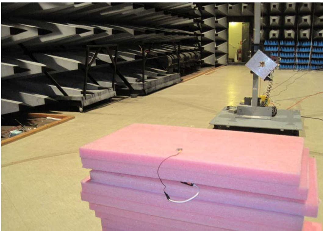
Photo 4.3.7 Test setup regarding measurement of radiated emission.
