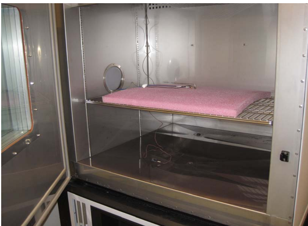
Photo 4.5.8 Test setup regarding measurement of 20 dB bandwidth.
