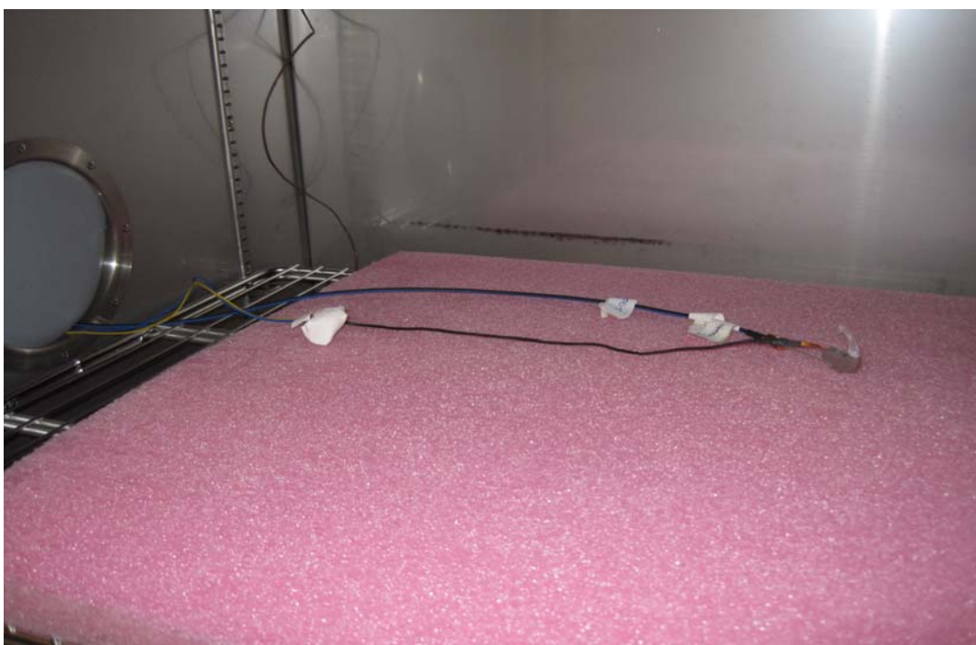
Photo 4.7.12 Test setup regarding measurement of occupied bandwidth, IC.
