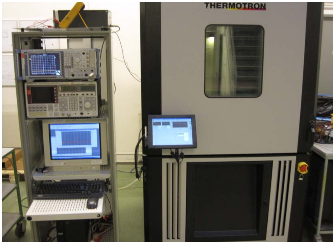
Photo 4.5.9 Test setup regarding measurement of 20 dB bandwidth.
