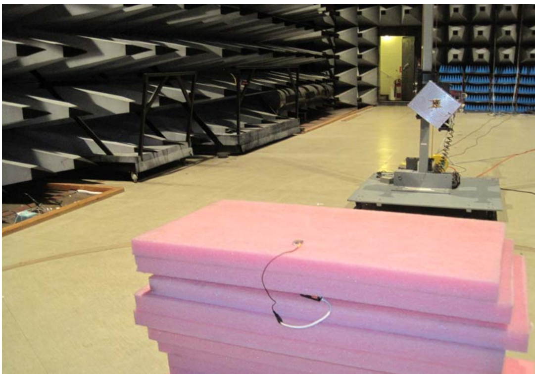
Photo 4.6.11 Test setup regarding measurement of band edge compliance.
