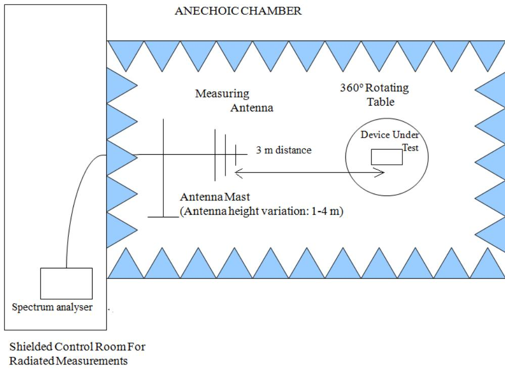
Radiated measurements setup  $f > 1 \text{ GHz}$  up to 17 GHz:
