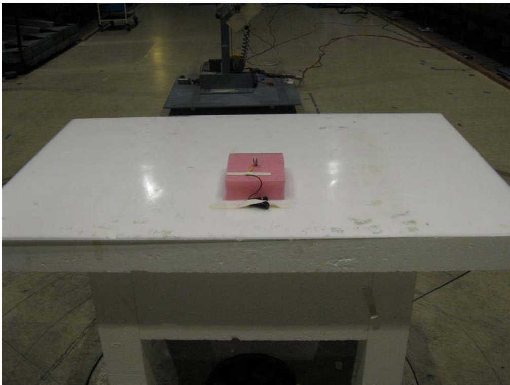
Photo 4.9.2 Test setup regarding measurement of field strength of fundamental.
