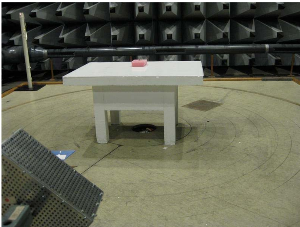
Photo 4.7.1 Test setup regarding measurement of radiated emission (above 1 GHz)
