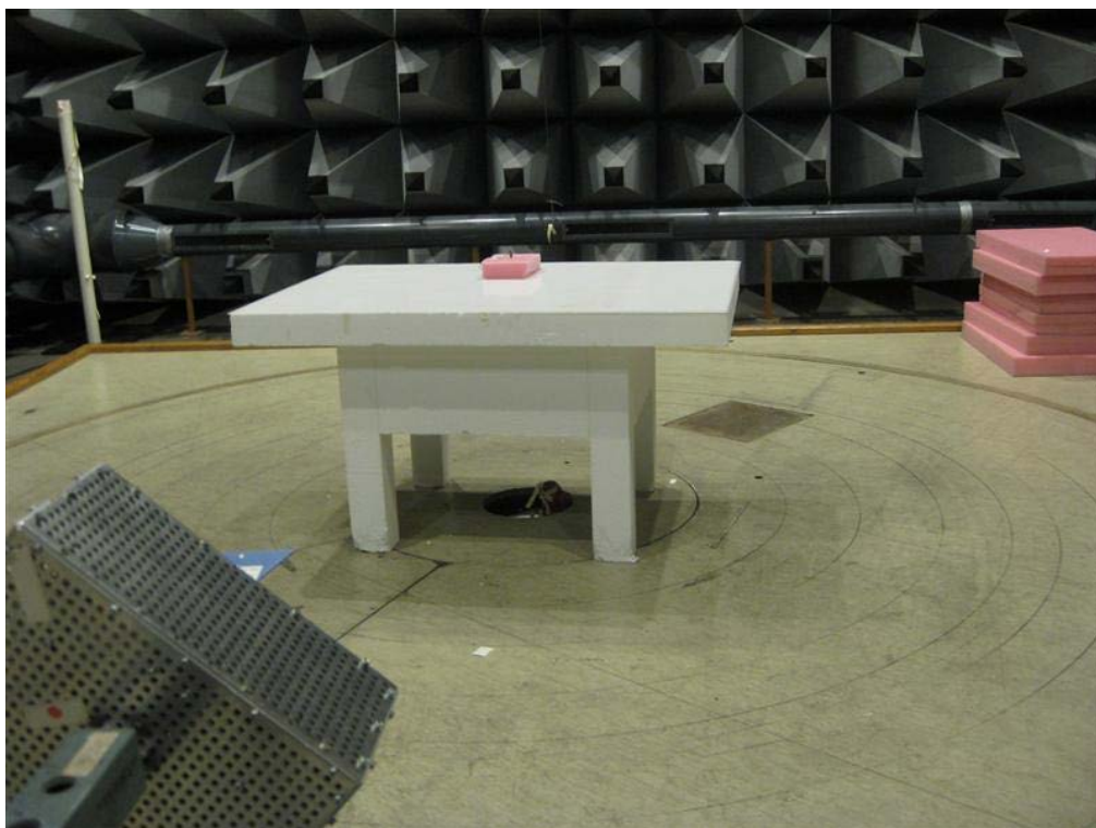
Photo 4.6.1 Test setup regarding measurement of radiated emission (above 1 GHz)
