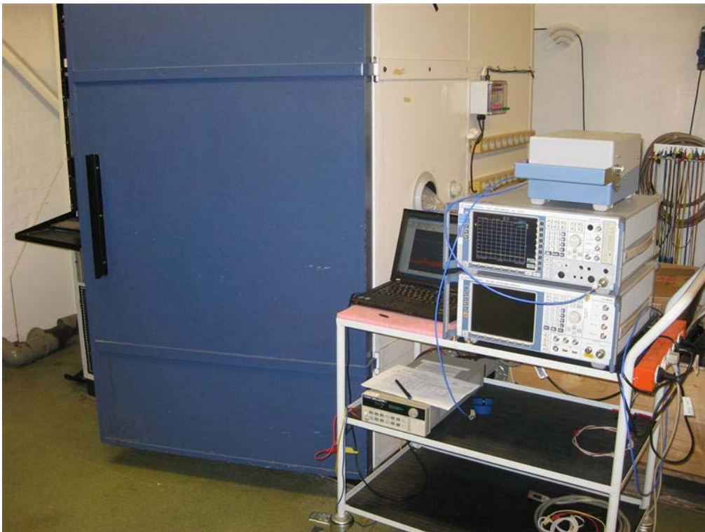
Photo 4.9.2 Test setup regarding measurement of 20 dB bandwidth
