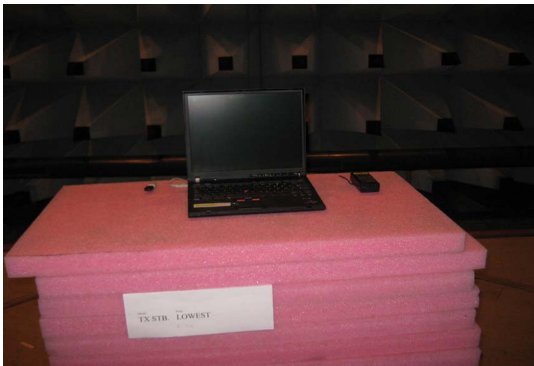
Photo 4.8.1 Test setup regarding measurement of field strength of fundamental.
