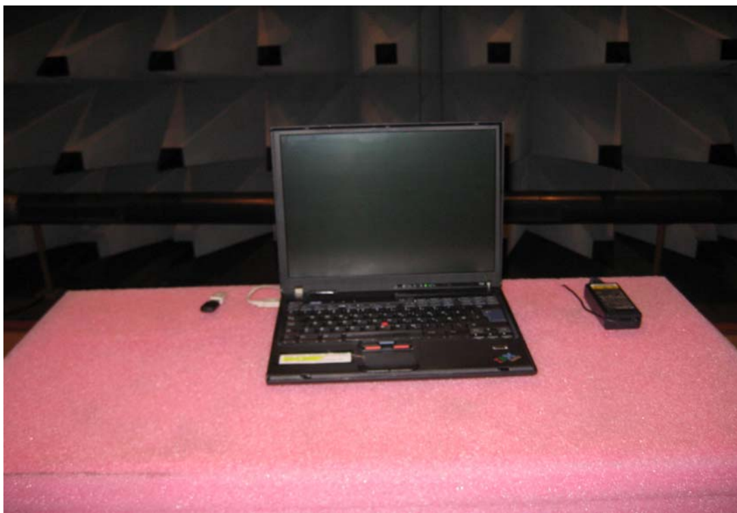
Photo 4.5.1 Test setup regarding measurement of radiated emission.
