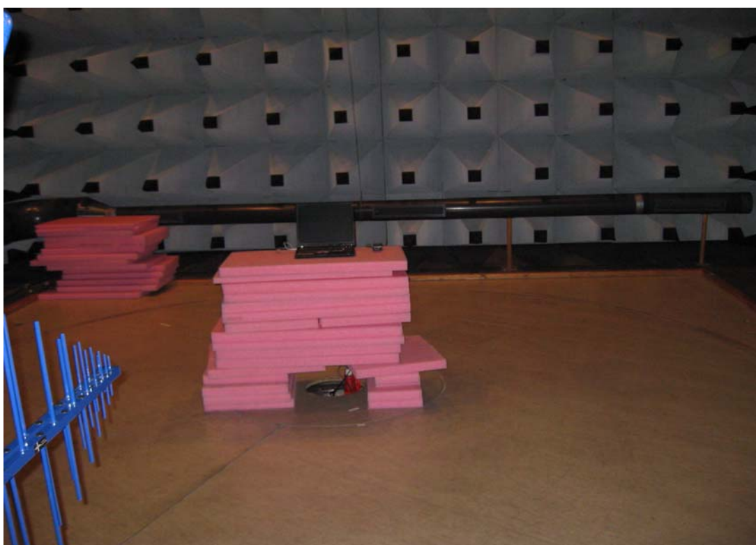
Photo 4.5.2 Test setup regarding measurement of radiated emission.
