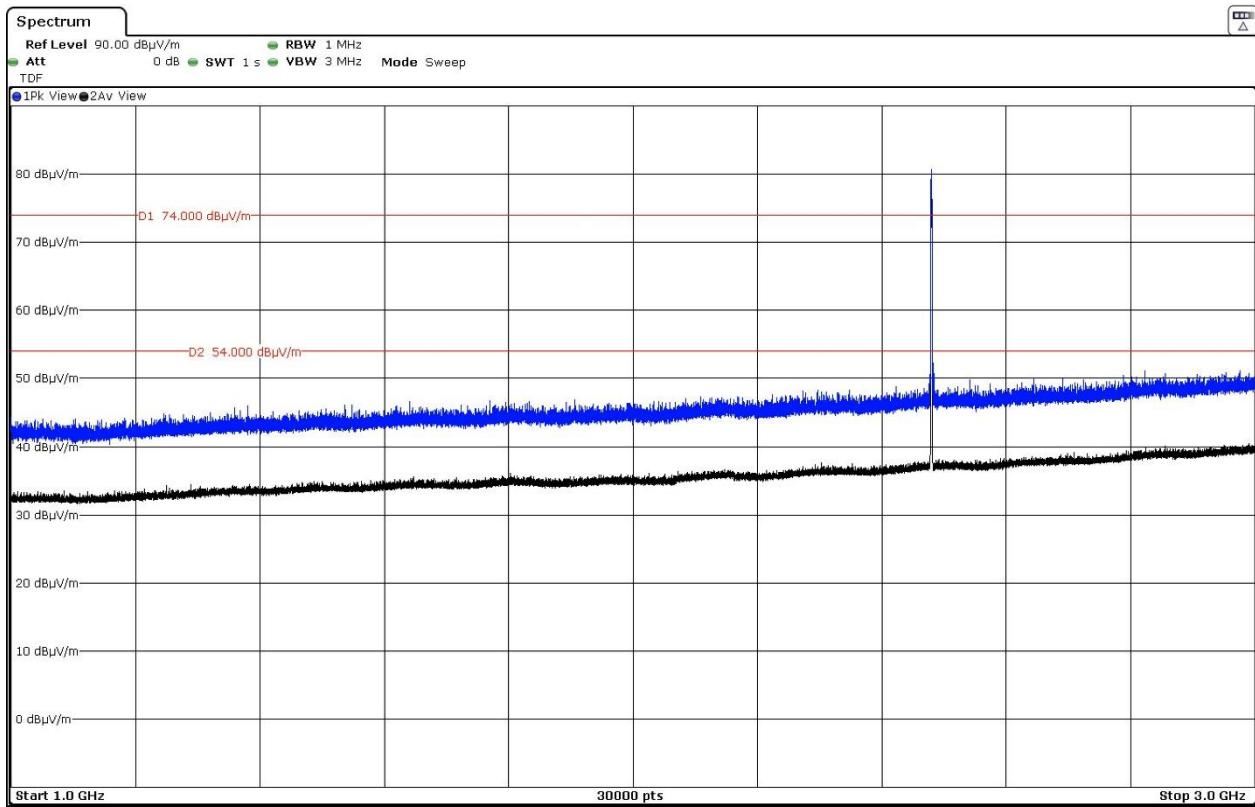
The peak above the highest limit is the Bluetooth LE carrier frequency.
