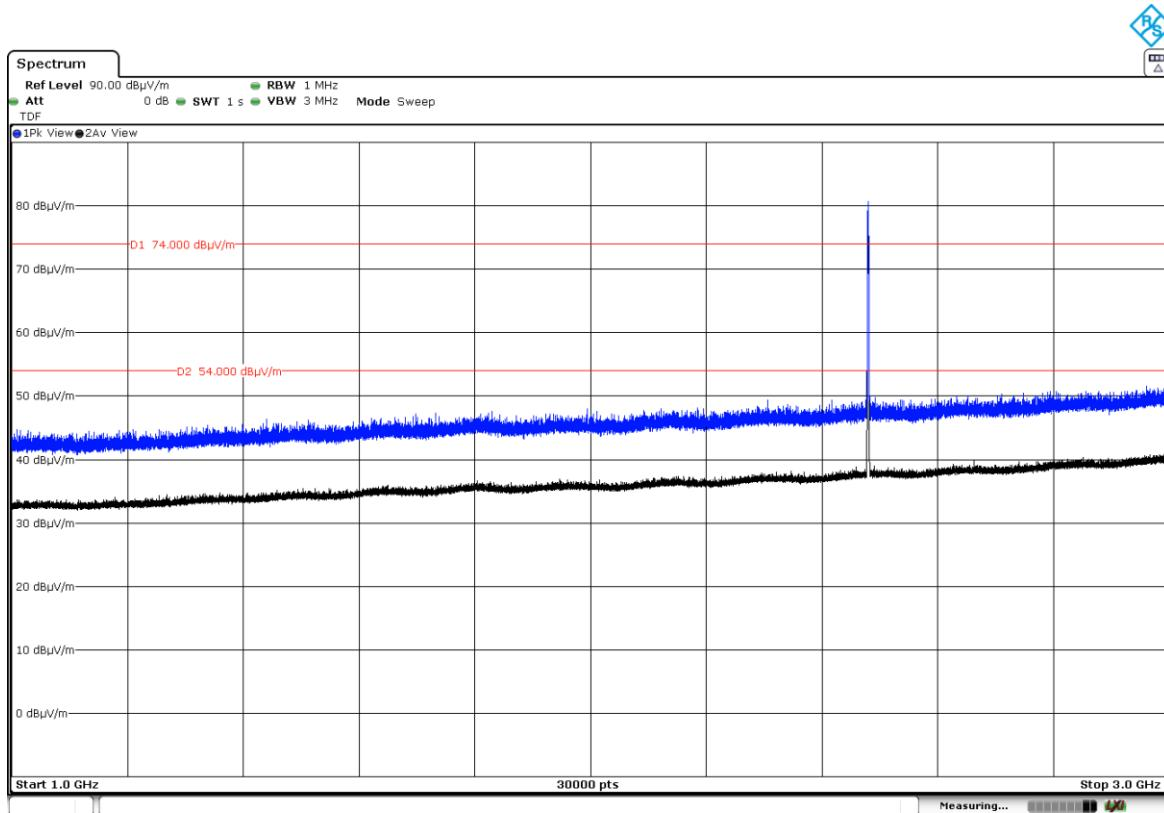
The peak above the highest limit is the Proprietary protocol 2.4 GHz carrier frequency.
