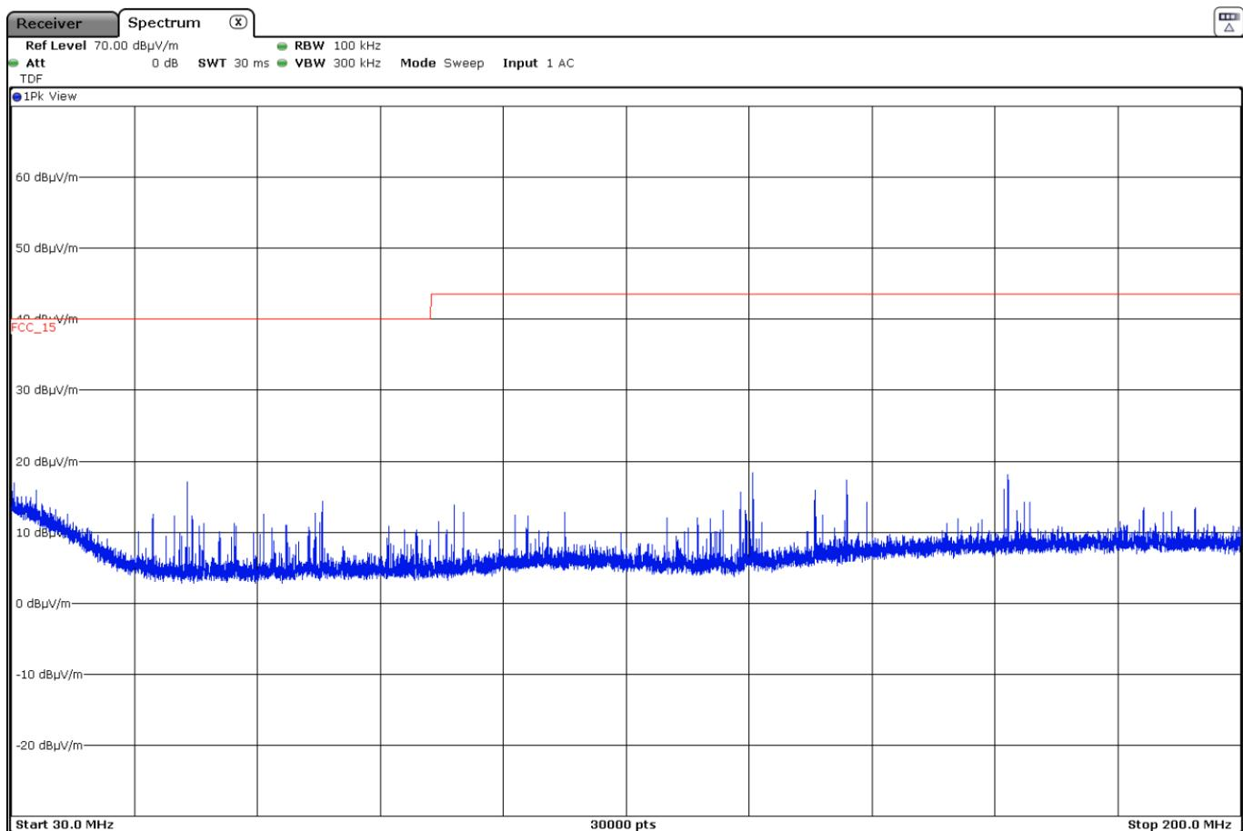
Note: The scan is performed with a peak detector.
