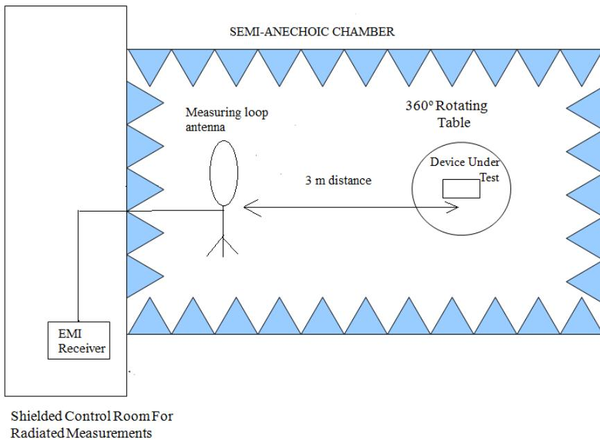
Radiated measurements setup  $f > 30$  MHz up to 60 MHz:
