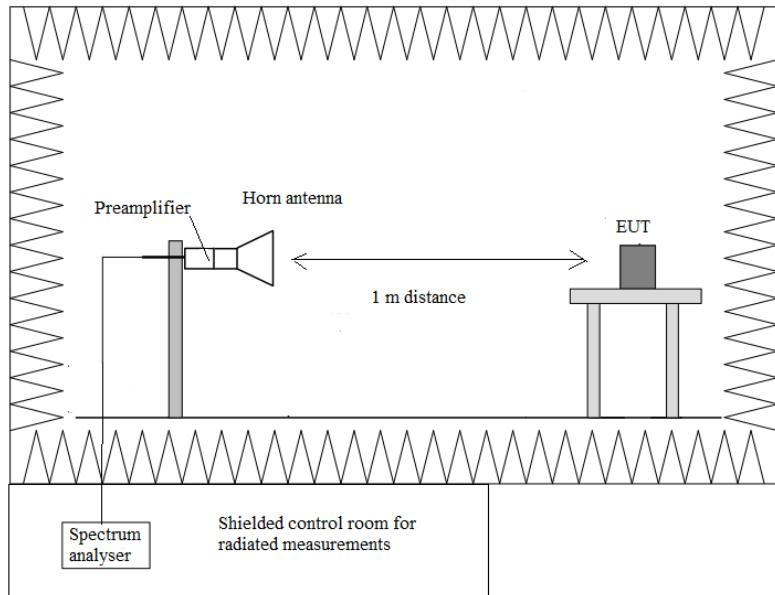
Radiated measurements setup  $f > 17$  GHz up to 40 GHz:
