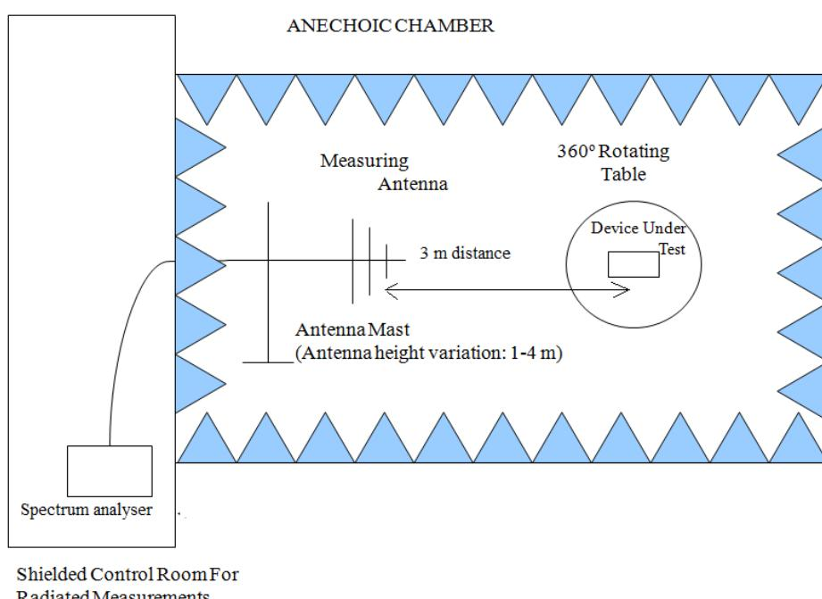
Radiated measurements setup  $f > 1$  GHz up to 17 GHz:
