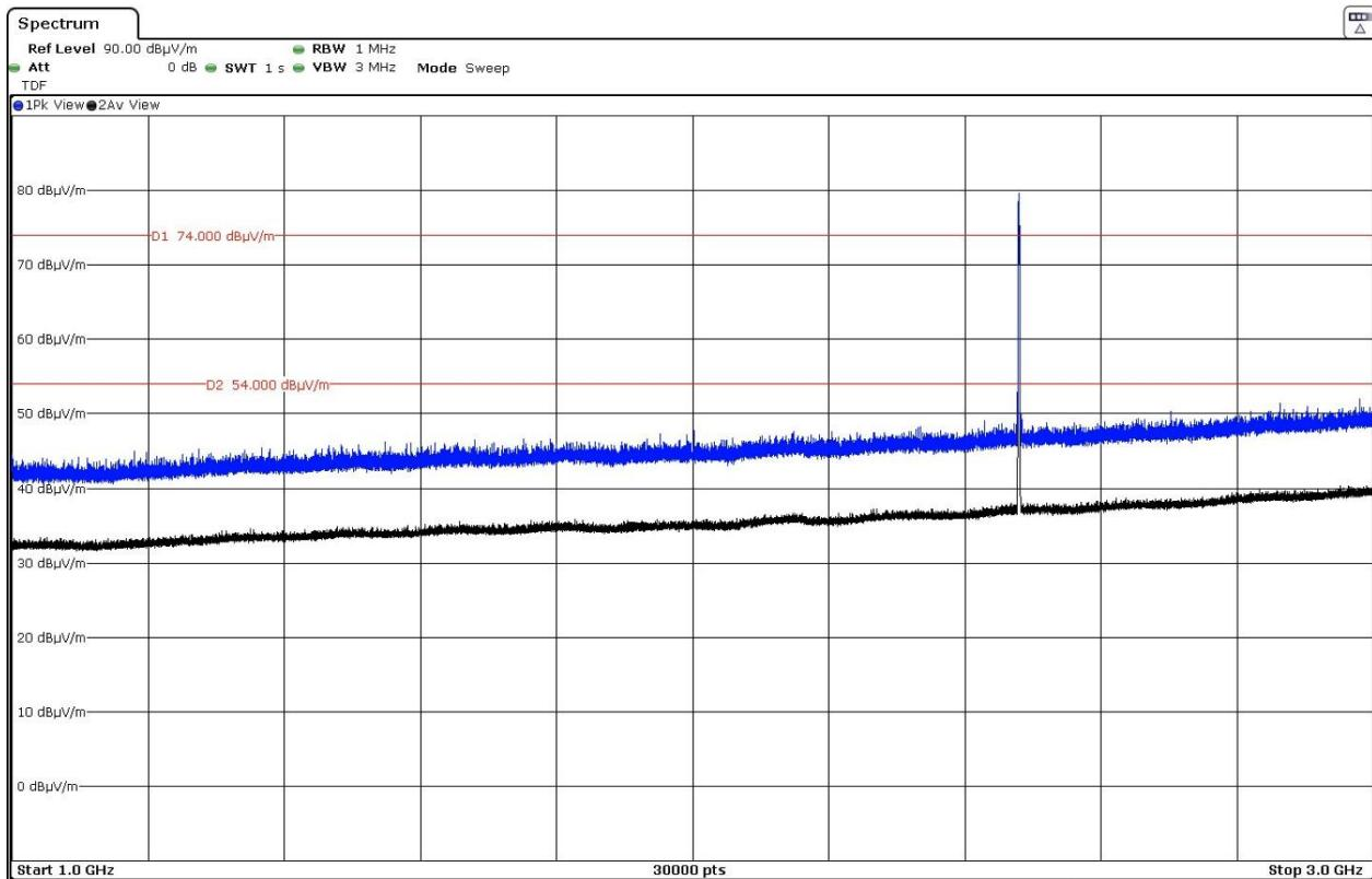
The peak above the highest limit is the Proprietary protocol 2.4 GHz carrier frequency.
