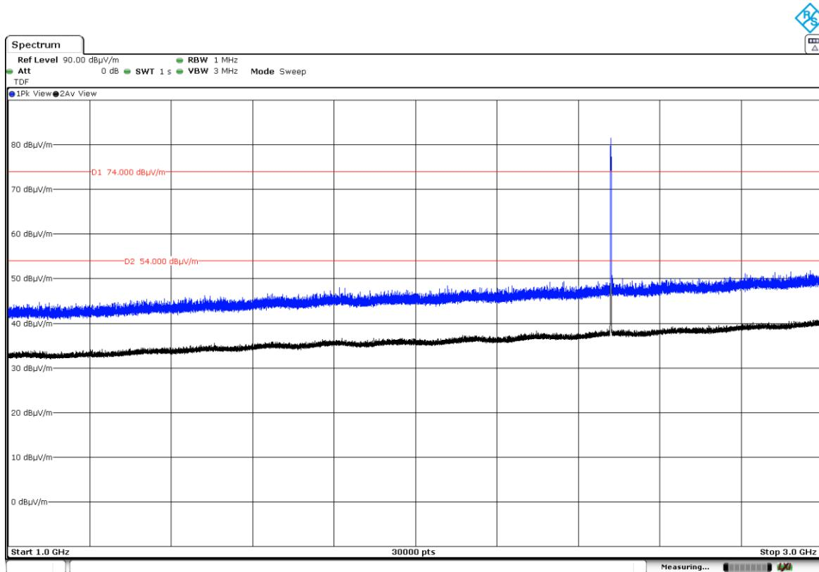
The peak above the highest limit is the Bluetooth LE carrier frequency.
