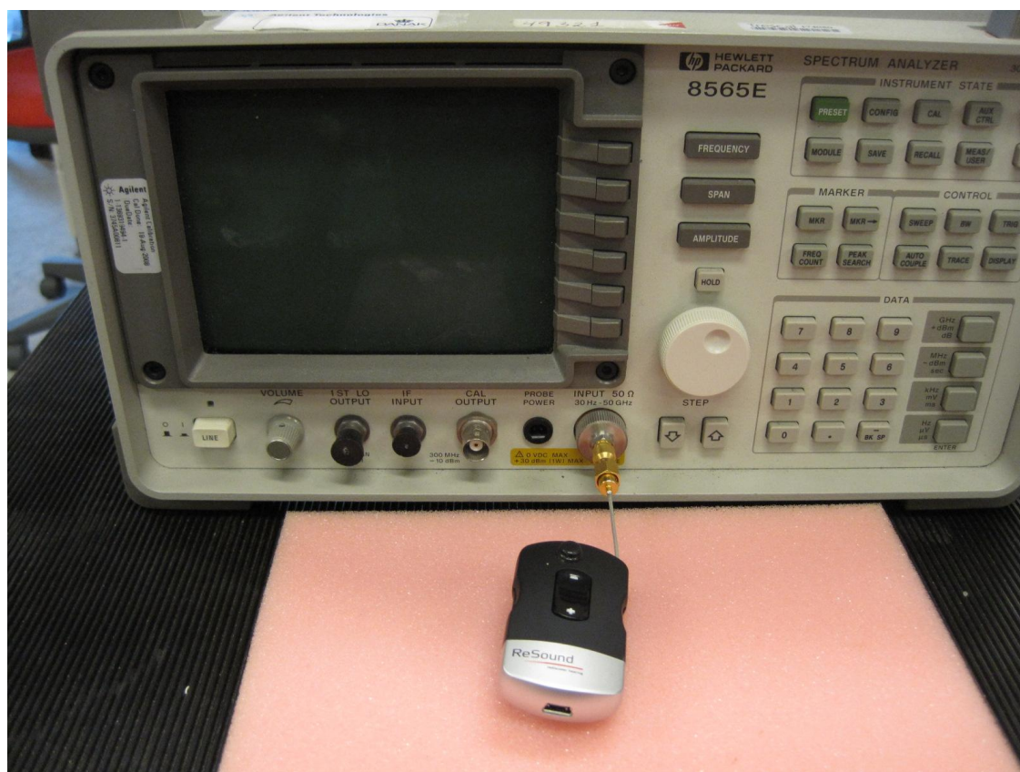
Photo 4.15.1 Test setup regarding measurement of power spectral density
