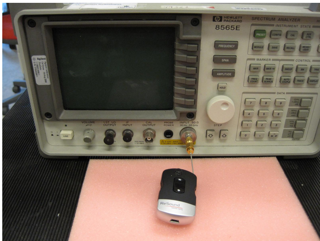
Photo 4.12.1 Test setup regarding measurement of peak output power, conducted
