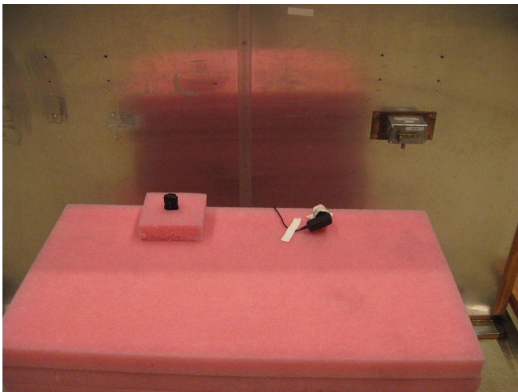
Photo 4.2.1 Test setup regarding measurement of radio frequency voltage on mains.
