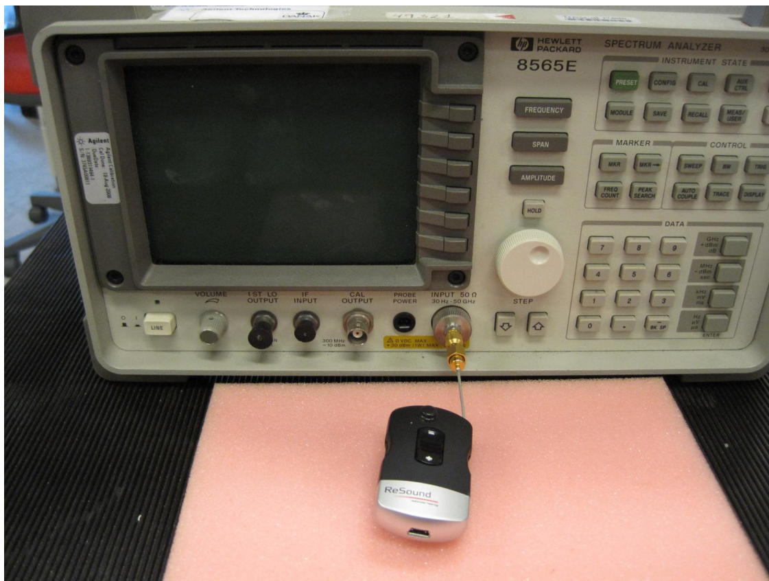
Photo 4.14.1 Test setup regarding measurement of band-edge compliance of RF conducted emissions
