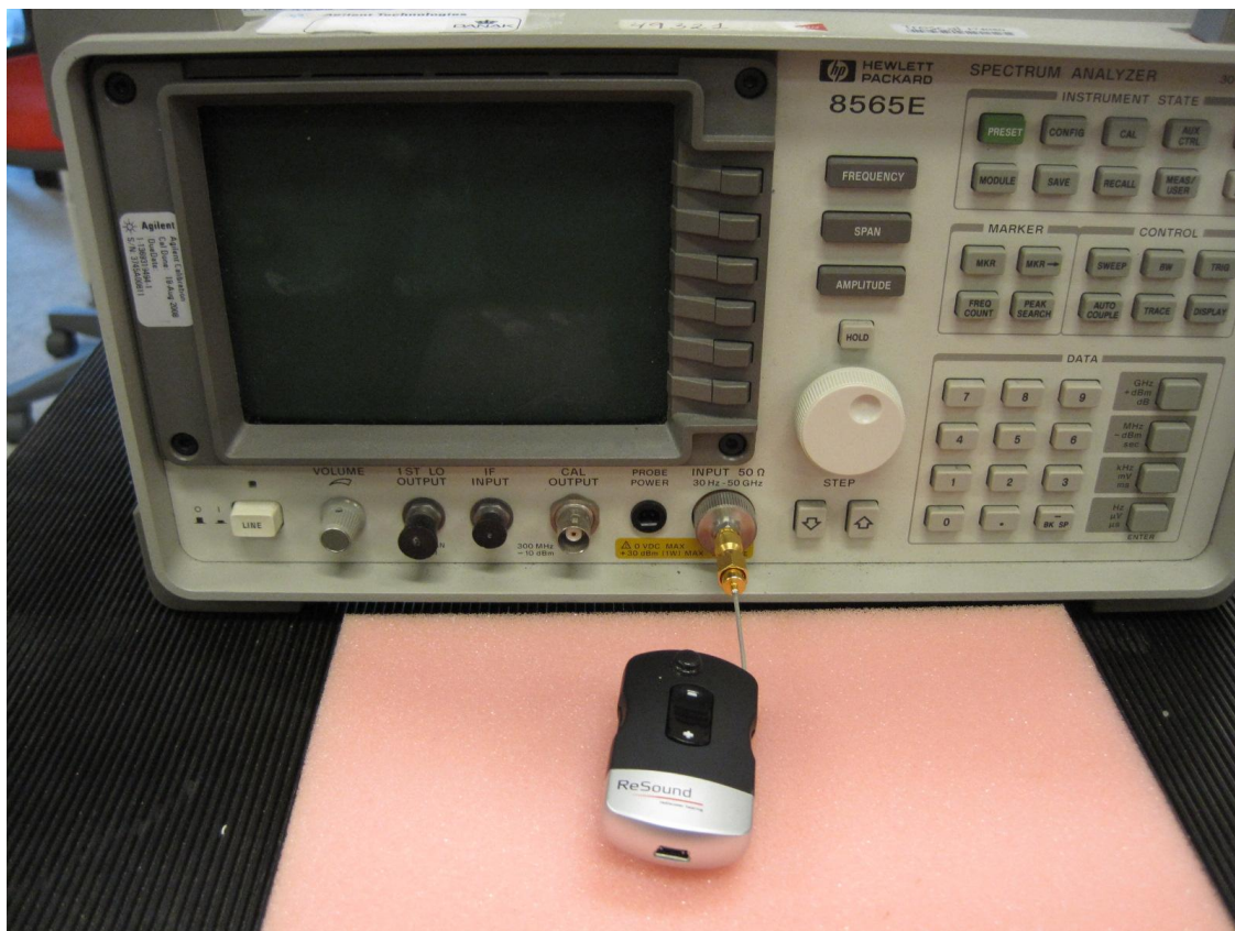
Photo 4.13.1 Test setup regarding measurement of Spurious RF Conducted Emissions
