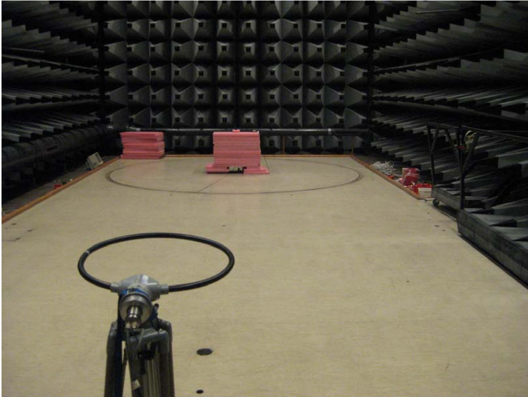
Photo 4.5.1 Test setup regarding measurement of radiated emission, 0.009 MHz to 30 MHz.
