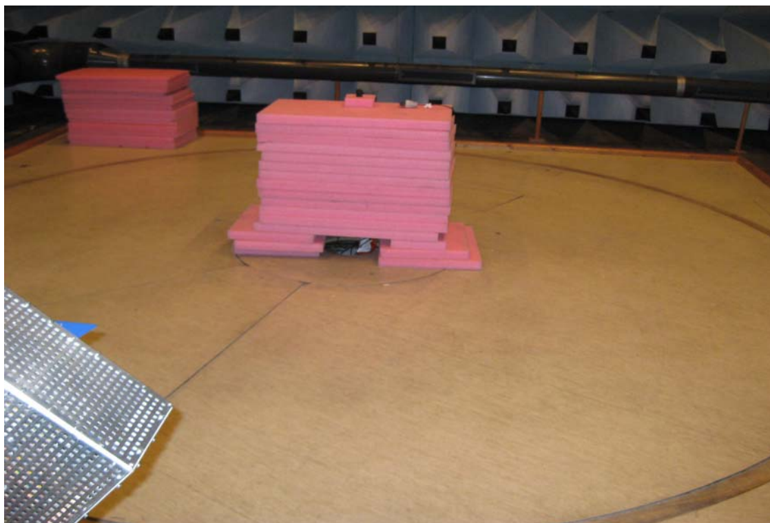
Photo 4.7.1 Test setup regarding measurement of radiated emission, 1 GHz to 25 GHz.
