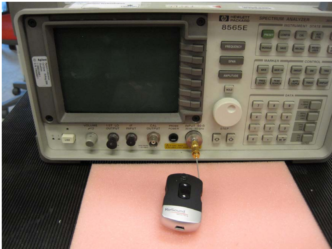
Photo 4.8.1 Test setup regarding measurement of 20 dB bandwidth and 6 dB bandwidth.
