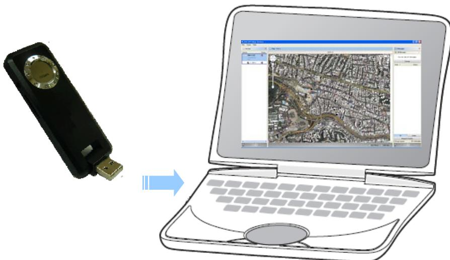
! For connecting SMS Server to PC, JOA USB Driver should be installed in your PC. Driver is in the provided installation CD or you can download from our website.
